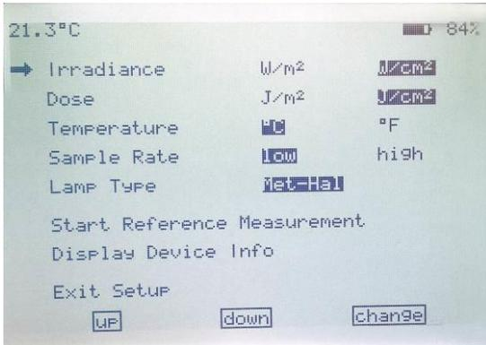
In the setup menu, you can also start a reference measurement and display the device info; i.e., wavelength band, serial number, firmware version, date/time, next calibration date, internal temperature.
