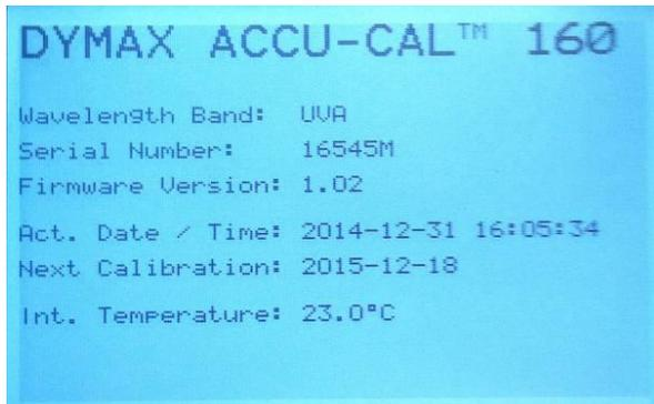
**Figure 3. Text Mode Screen - Push the Middle Button to Enter Setup**
